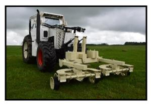
The Armtrac Roller System is designed to protect vehicles from the effects of victim operated devices and provides a level of confidence when proving routes for the presence of mines and IEDs. It can be used at up to 50 KPH when fitted to the Armtrac 100 and at lower speed with tracked Armtrac vehicles but another self-weight version of the Roller System can also be used with APCs or MBTs.
