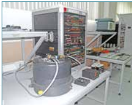
Anti-ice System Repair Test Stand
