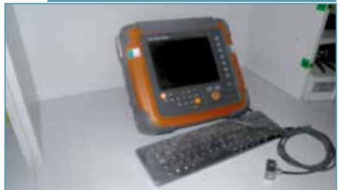
IMPROVED ULTRASONIC PHASED ARRAY
