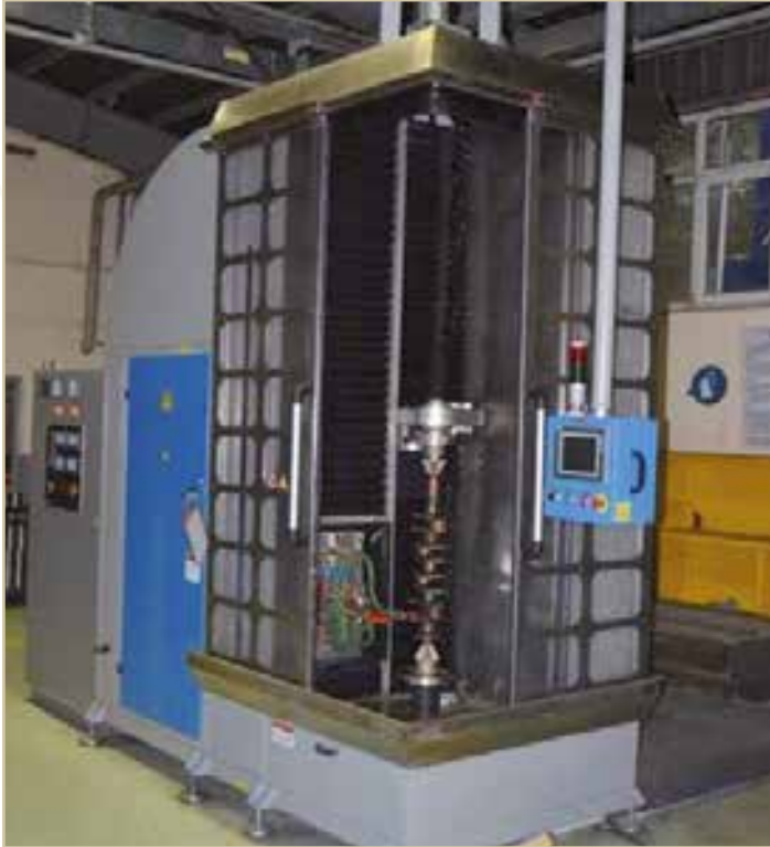
■ HARDENING WITH INDUCTION MACHINE
