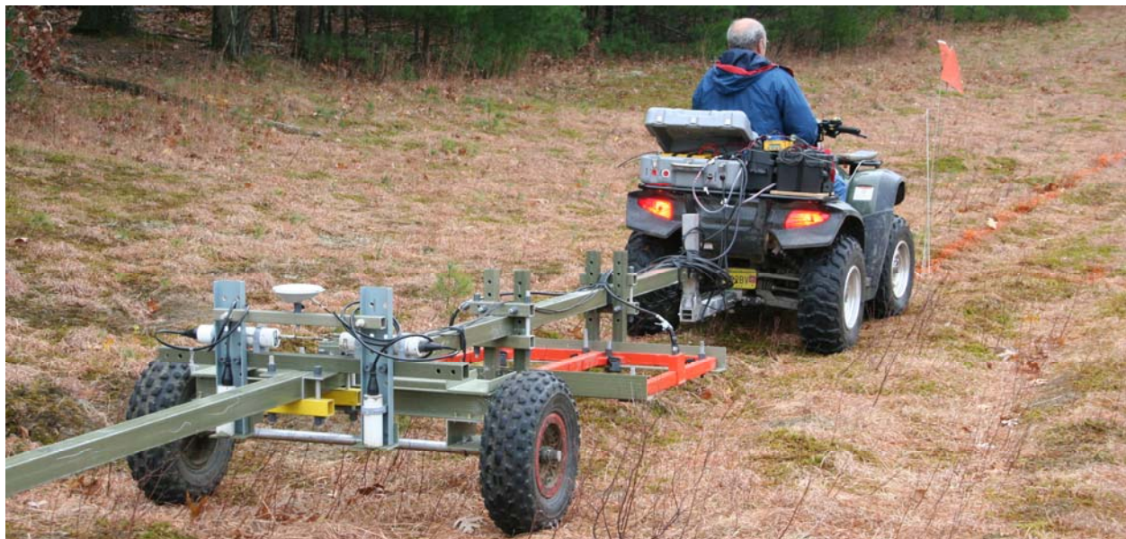
Figure 41: "TSEMS" using MPI box, two magnetometers and two EM61s, towed by an ATV
