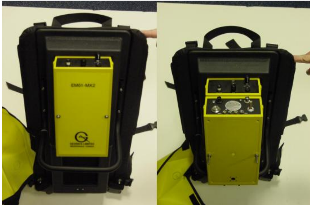
Figure 2: COTS EM61 backpack with standard COTS EM61 electronics (left), and with additional MPI box mounted on top of EM61 box using through-holes (right)
