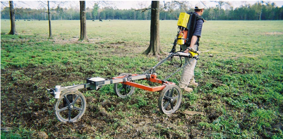
Figure 36: MSEMS cart, with relocated battery and GPS, pulled over rough terrain at Camp Sibert Site 8
