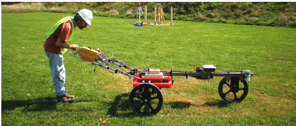
Figure 37: MSEMS utilizing an EM61 Mk2A with no backpack as part of testing of a Simplified Combined EMI and Magnetometer Prototype (SCEMP) for NVESD HD division
