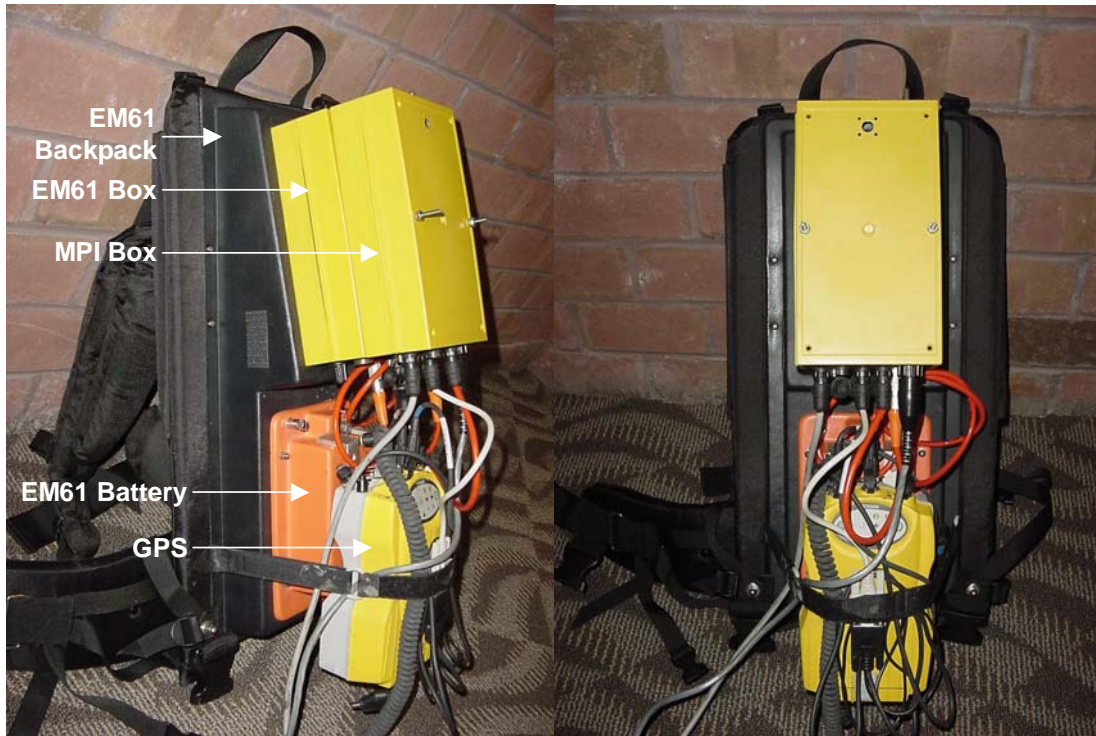
Figure 3: Close-ups of EM61 backpack with EM61 electronics box, EM61 battery, MPI box, and GPS. The GPS is strapped to the backpack with a velcro strap, and has a right-angle bracket so it won't slide off the battery.
