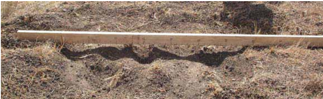
Figure 53. MV-4 Ground Profile Photographs, New Hammers, Mines at 10 cm DOB
