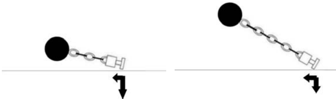
Figure 27. Shaft Height Geometry
